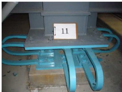
Test specimen of steel damper (removed)
